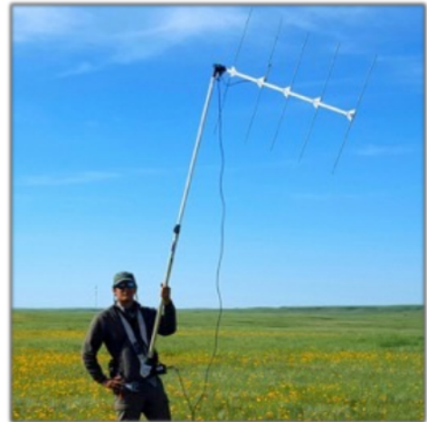
Figure 6: Bird Conservancy crew lead Sasha Robin with 5-element antenna and extension pole, used to track tagged birds. Photo by N. Guido.
